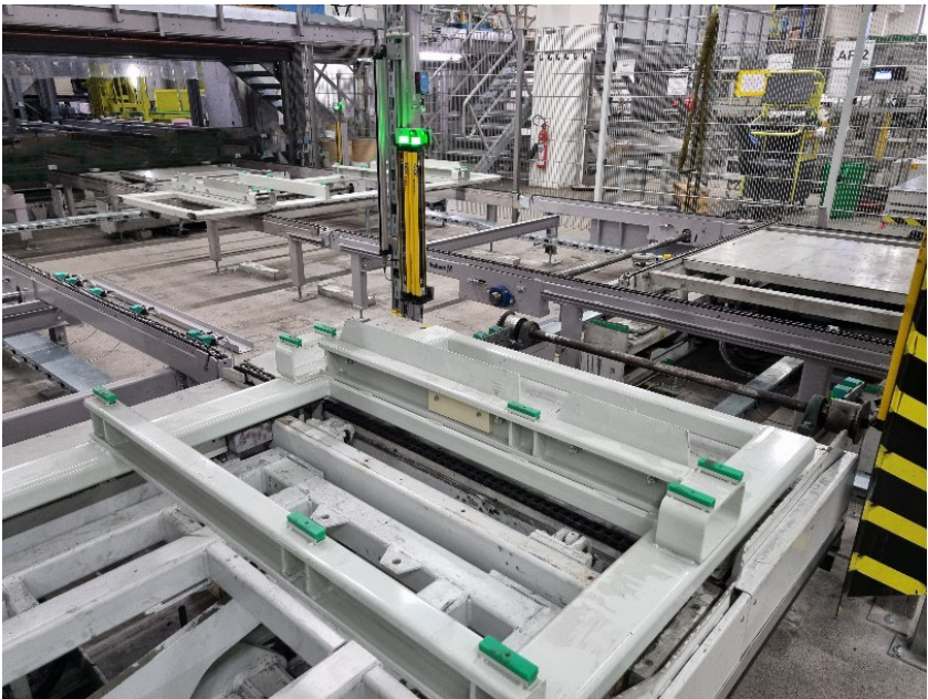
Image 2 - Chain cross-conveyor expanded Together with Vollert, the existing chain cross-conveyor was, therefore, expanded by four additional buffer stations to create capacities for future performance increases. This makes it possible to buffer skids up- and downstream of the workstation.
