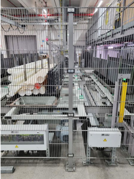
Image 1 - Chain cross-conveyor before Bottleneck in production. Too-short conveyor sections in an existing chain cross-conveyor kept causing delays and waiting times in storage and retrieval of a high-bay warehouse at Ensinger.
