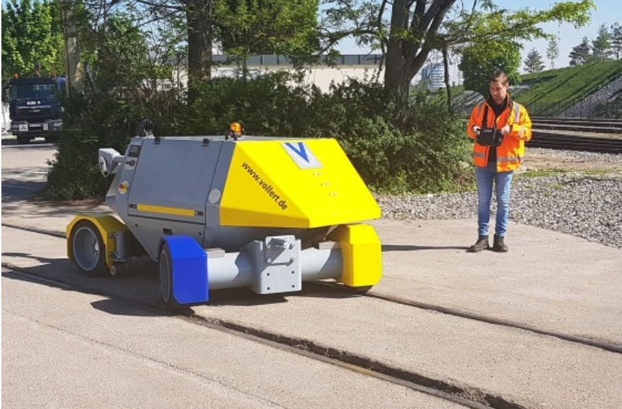
Image 3 The articulated steering is controlled by the speed control of the wheel hub motors with turning radiuses of only 7.2 m that are gentle to the tires and low-wear and even a 360° turn on the spot.
