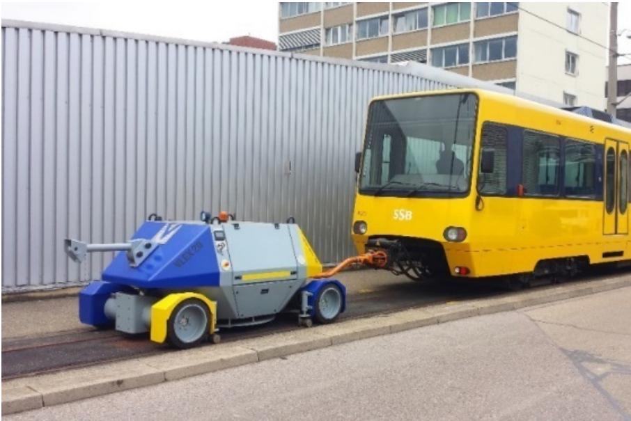
Image 4 The vehicle masters smaller obstacles as well as chuckholes without any loss of structural stability and traction even on unpaved but load-bearing surfaces. The road-rail robot is versatile.
