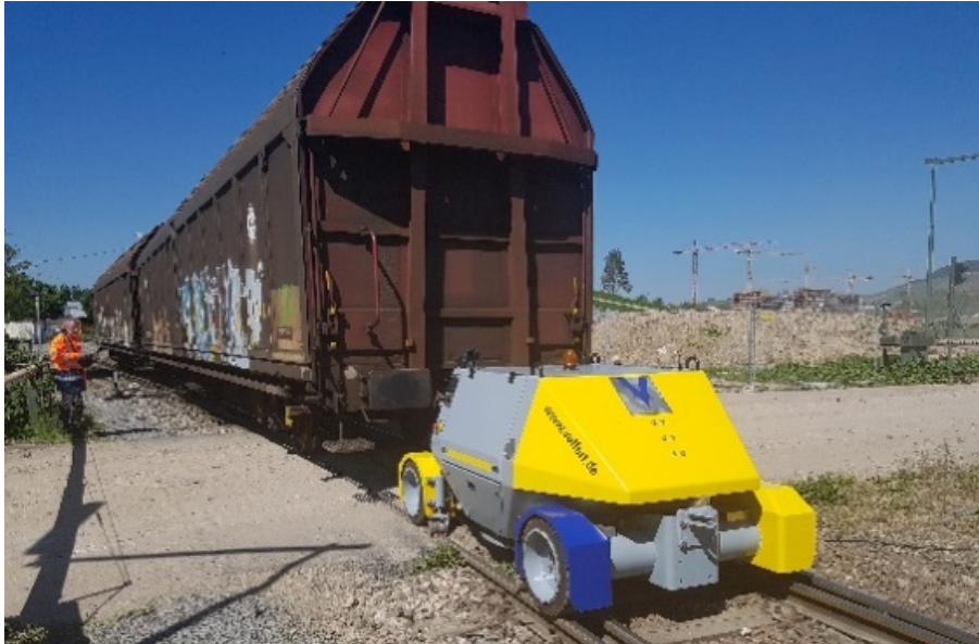
Image 1 Compact, flexible, battery-driven and exhaust-free: Vollert's innovative VLEX road-rail robot is the optimal solution for easy shunting operations of up to 300 tons on rail and road.
