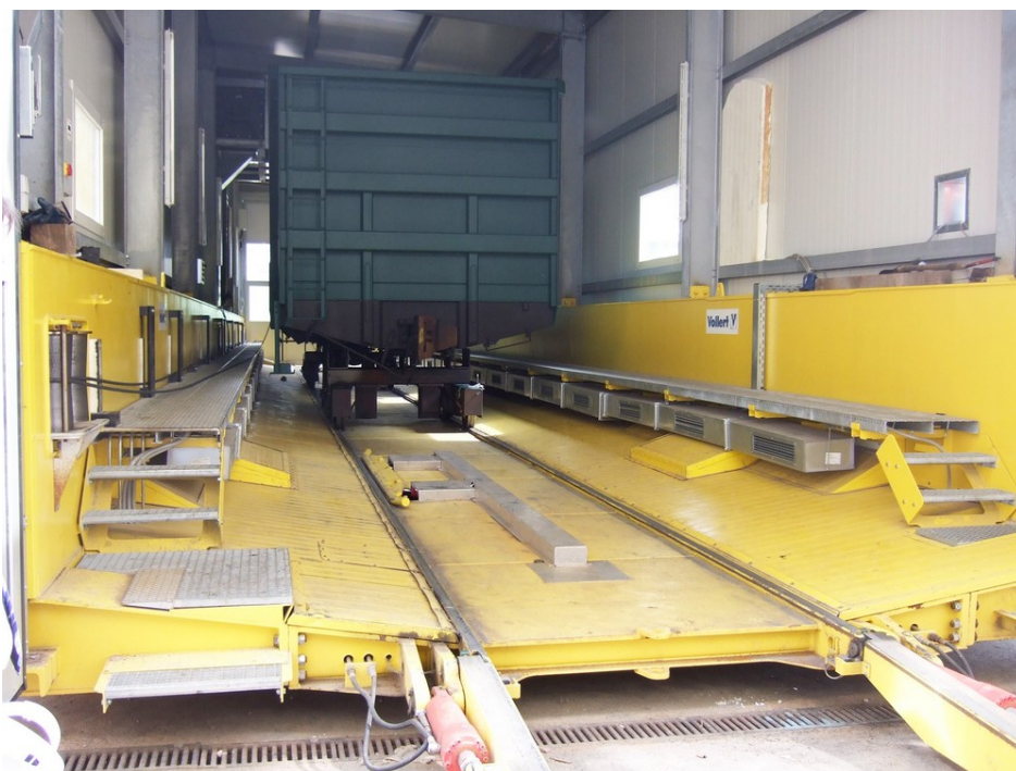
Image 3 Heavy-duty transfer cars from Vollert, with heated, full enclosures, optimally protect the railway carriages from the elements so that they can be coated efficiently in TVSZ's new plant in Russia.
