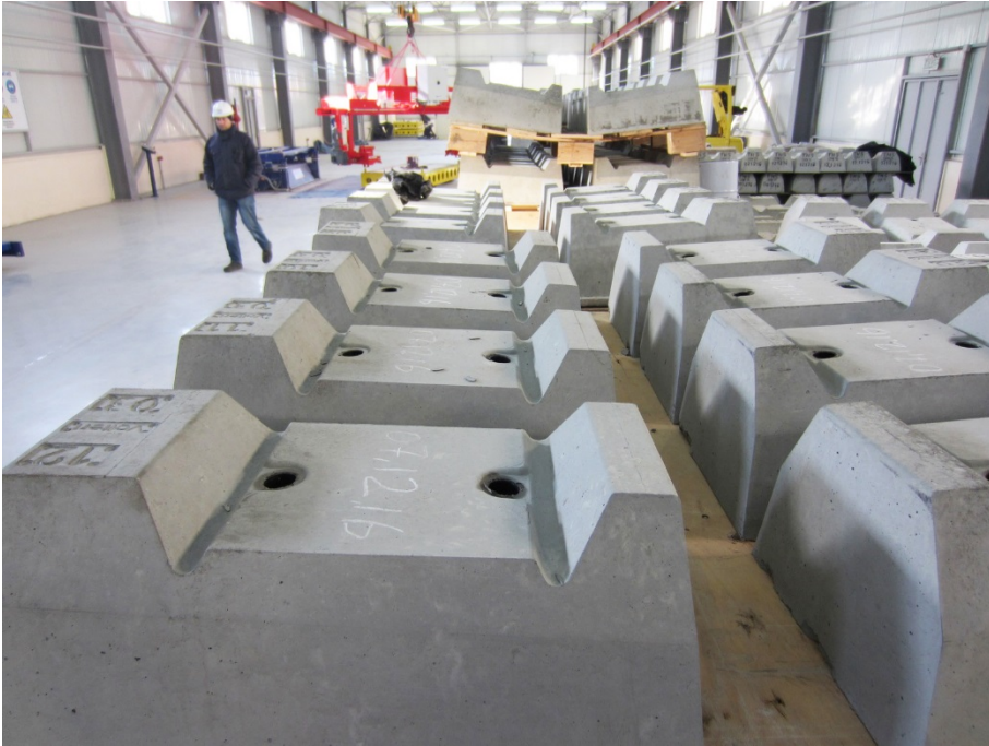
Image 5 With 20 moulds, up to 30,000 concrete sleepers can be produced per year in the concrete sleeper plant.
