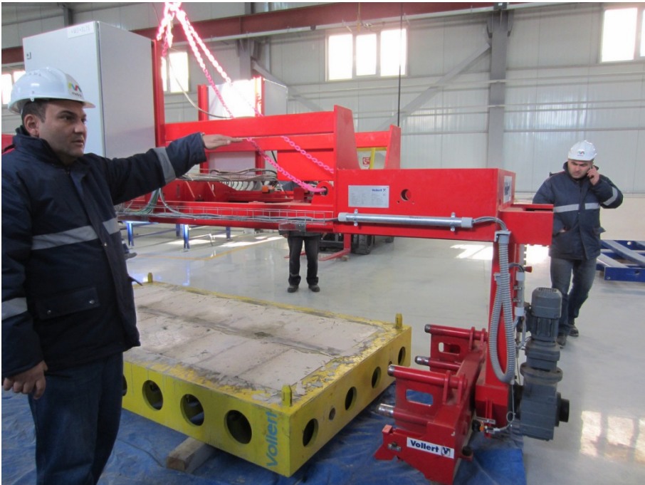
Image 4 The sleeper blocks are turned over with a turning manipulator and demoulded by an impact from a rocker disc.
