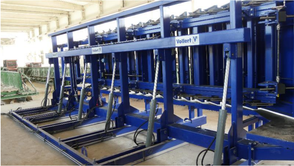
Image 1 Hydraulic KOMBISTEP stair formwork at Limelog in Hungary.
