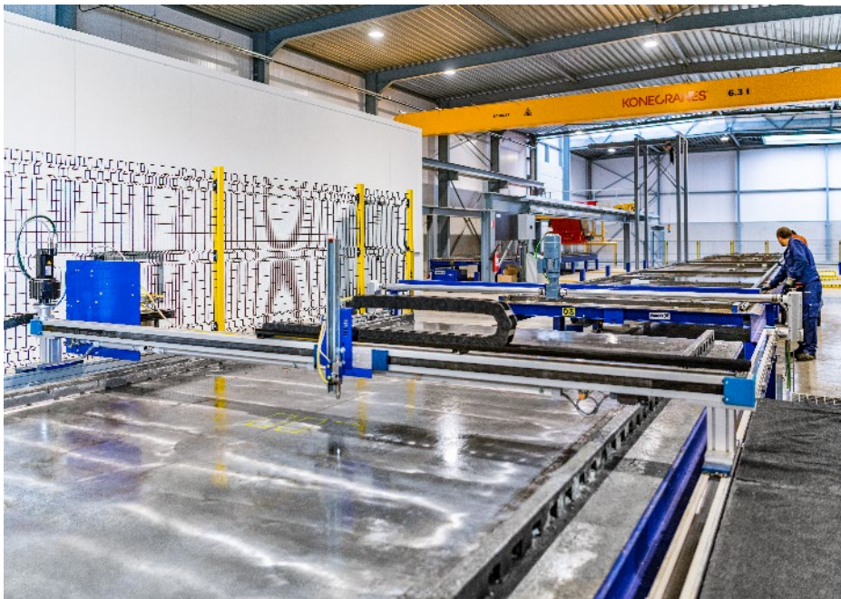
Image 2 For precise recording of the contours of the ceiling parts, a SMART PLOT plotter applies colour according to CAD/CAM specifications.
