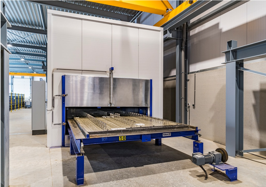
Image 5 Another technical highlight: the fully insulated VARIO CURE curing chamber with two rack towers set in a row.
