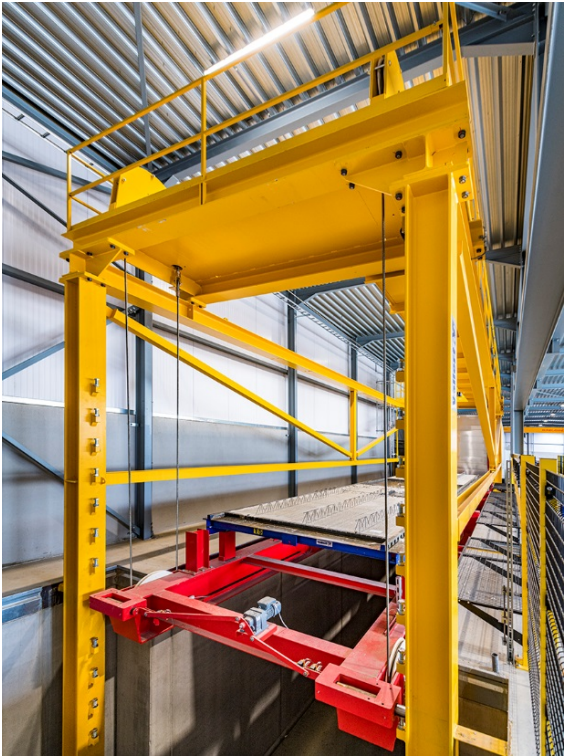
Image 6 The stationary VARIO STORE storage and retrieval machine takes over the floor slabs for storage and retrieval.
