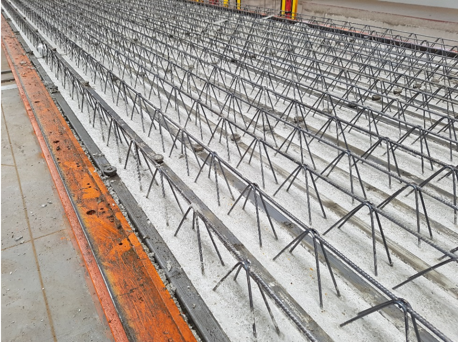
Image 6 The beams can be made up to 8 m long. Assuming a beam length of 3 - 4 m and up to 60 elements can be produced simultaneously.
