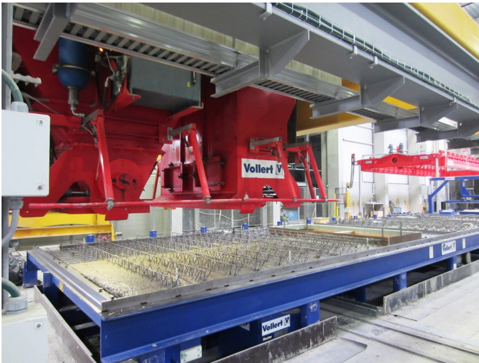
Fig. 4: The twin concrete bucket is a true novelty as well. This way, not only normal concrete can be applied but also coloured exposed concrete.
