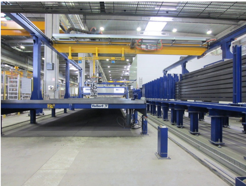
Fig.2: A SMART SET 2 shuttering robot places the RATEC shuttering profiles precisely onto the prepared circulating pallet at high movement speeds
