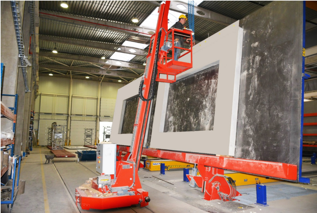
Fig. 7: The solid concrete and semi-finished parts are vertically lifted off by a Vario TILT high-performance tilting station
