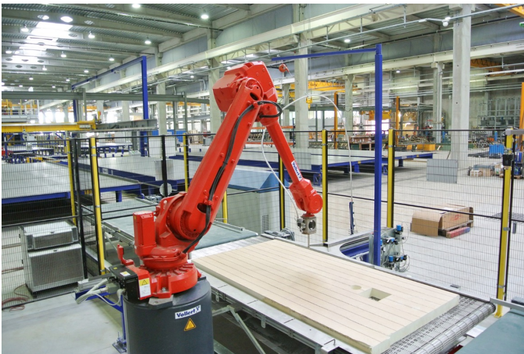
Fig. 6: For the production of sandwich concrete parts the new Cordeel factory relies on the ISO-MATIC 2.0, which permits highly precise and fully automated preparation of insulation
