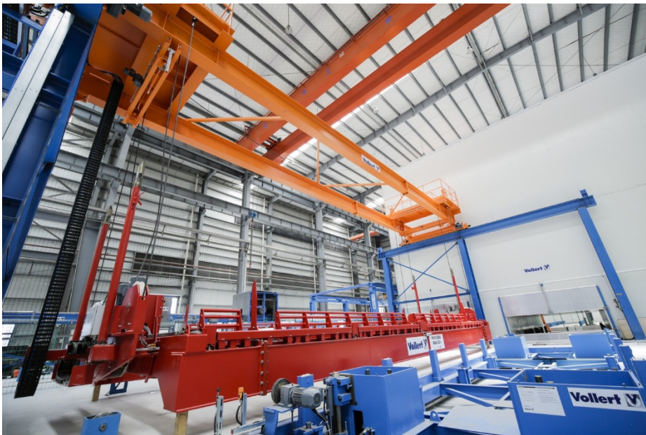
Fig. 6: State-of-the-art VARIO TURN pallet turning equipment for double-wall production
