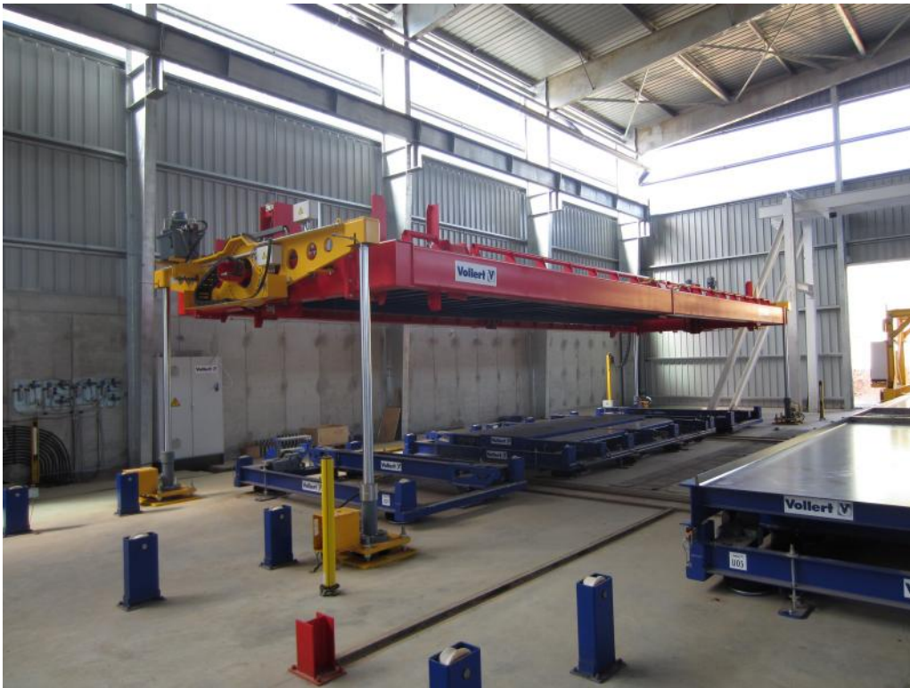
Fig. 7: Double wall production with stationary pallet turning device
