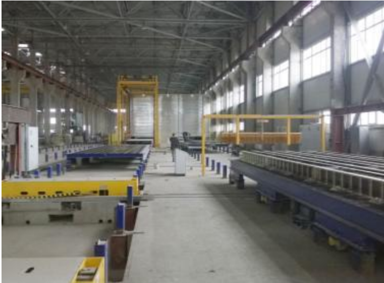
Fig. 3: Vollert has developed special processes for the production of sandwich walls and uses intelligent transverse transport technology for this
