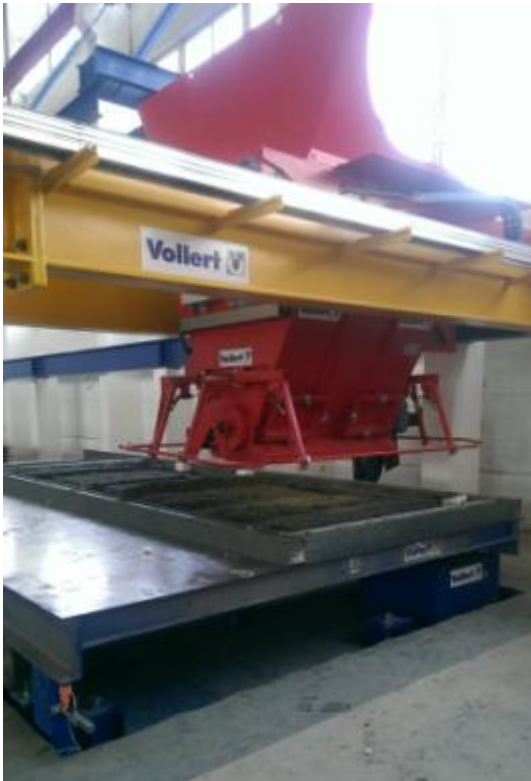
Fig. 11: Hydraulically actuated flat slide valves and a spiked roller apply the concrete precisely and evenly at a total of four concreting stations.
