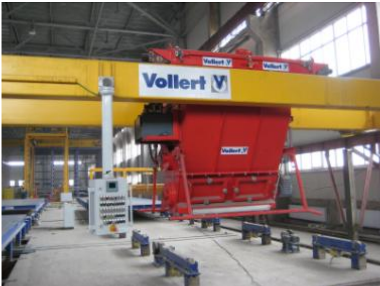
Fig. 4: A semi-automated concrete distributor applies the concrete evenly and with high precision
