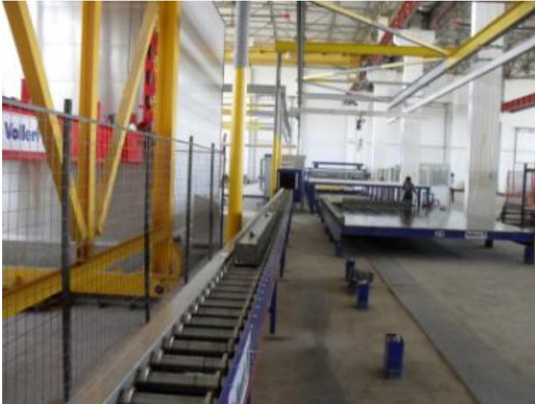
Fig. 10: Thorough pallet and shuttering preparation is indispensable for the production of high-quality precast concrete elements
