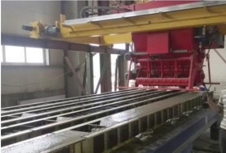
Fig. 5: A discharge area of up to 3.20 m is achieved with the aid of a bridge bogie
